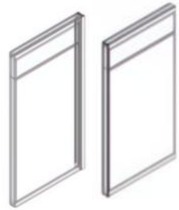
WALL STARTER & END TRIMMING
